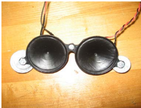
Figure 1 Waterproofed loudspeakers serving as hydrophones
