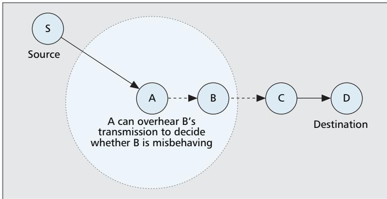
■ **Figure 2.** Watchdog mechanism for MANETs.
