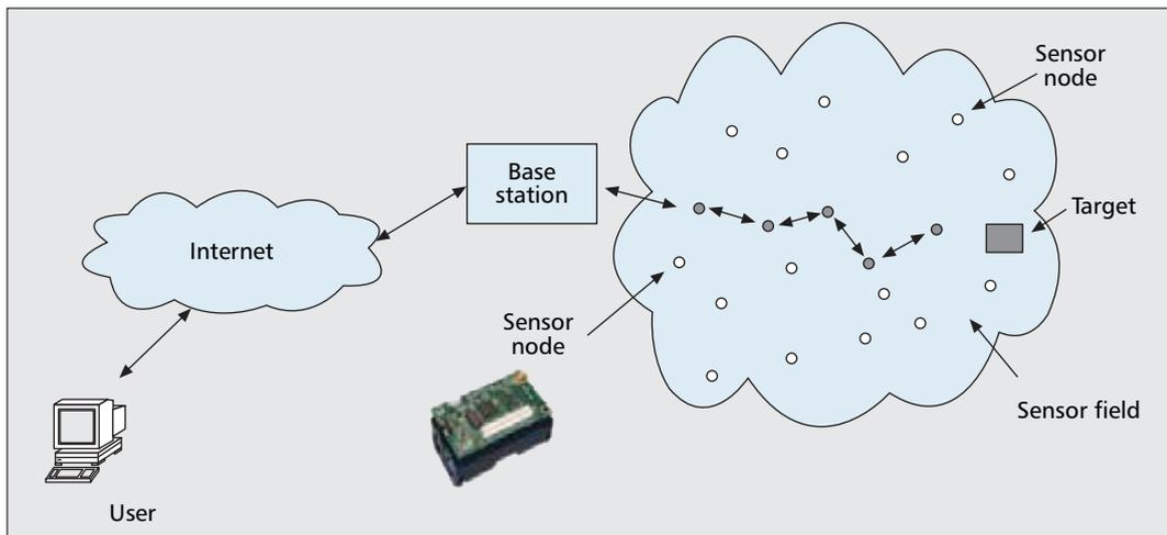
■ **Figure 1.** An example of a wireless sensor network.
