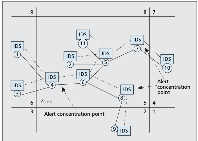
■ **Figure 3.** The zone-based intrusion detection system for MANETs.
